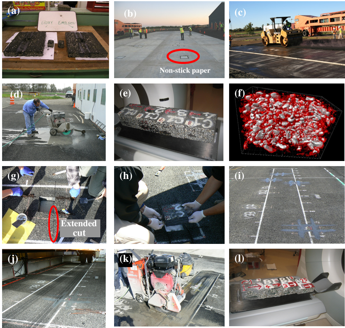
Figure 6.1 The general procedure followed for CT image data collection (before-after HVS testing).
