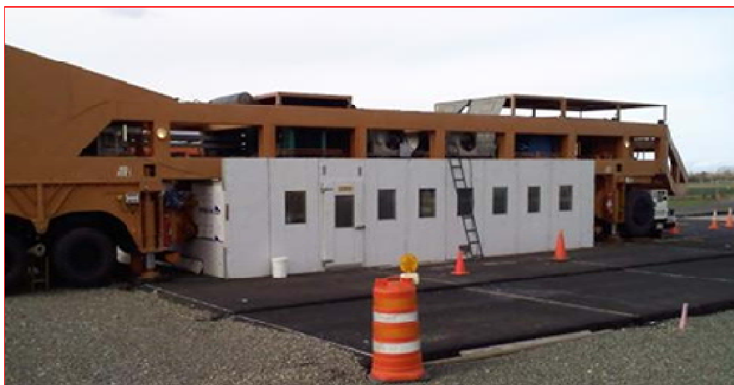
Figure 2.2 Specifications and photograph of HVS.
