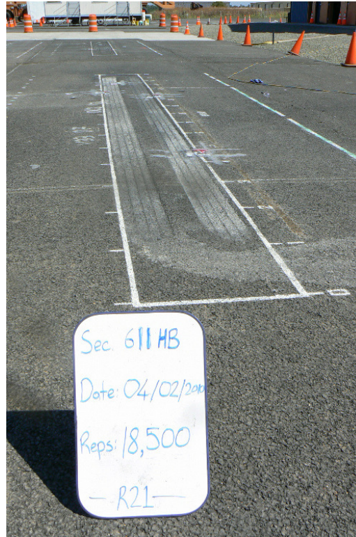
Figure A.34 611HB - RHMA-G - 114 mm: Section photograph at test completion.
